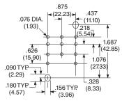
\_\_27E046 HAS TERMINALS .144" (3.66 mm) LONG. 27E305 HAS TERMINALS .184" (4.67 mm) LONG.
